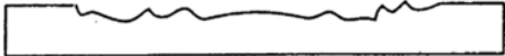
SCULPTURED DIE, a hand tooled brass die containing many levels at varying depths.
